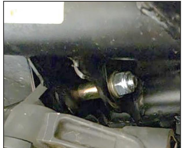
**Note: Position the shock eyelet so that it is closest to the front of the vehicle and the lock nut is always facing towards the rear.**
