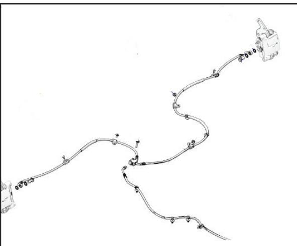
Bend up or drill out the factory p-clamps until they snap off, then remove the clamps.
