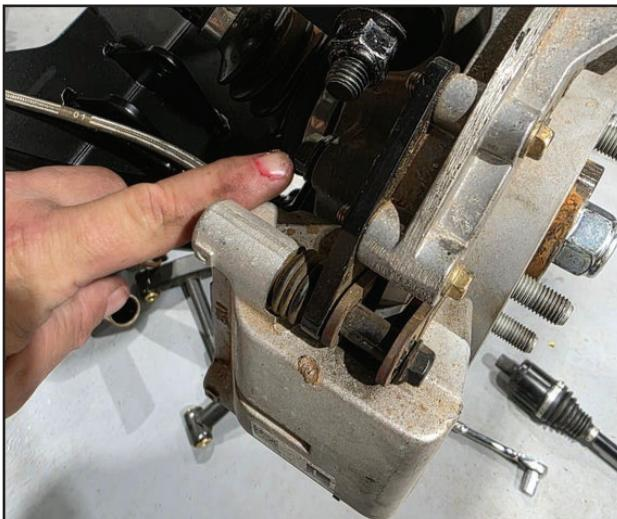
Attach the calipers back onto the hub assembly. Make sure to route the lines so that they do not come in contact with any moving parts.
