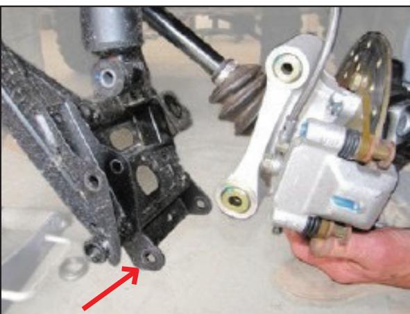
Disconnect the hub assembly from the arms. You will reuse the factory hardware to connect the new control arms to the frame.
