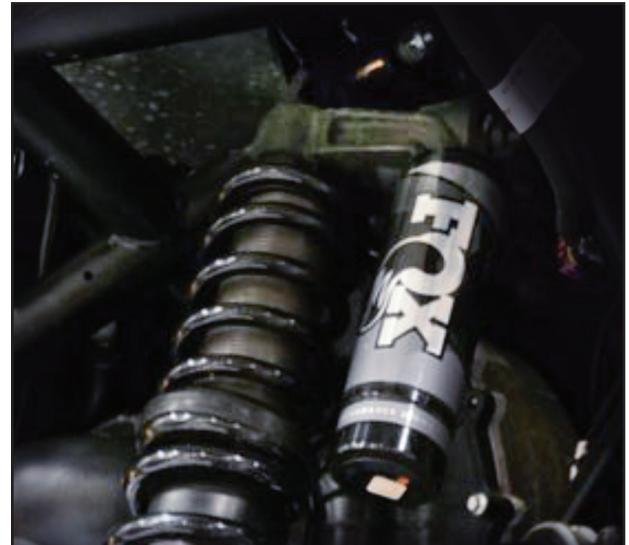
Connect the lower shock eyelet to the lower control arm with the factory hardware. Using the brake line clamps provided, secure the brake lines to the lower control arm. Ensure that the lines do not encounter moving parts.
