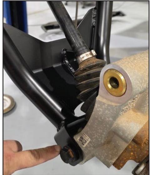
Attach the upper arm to the frame tabs and the hub assembly. Then attach the calipers back onto the hub assembly.
